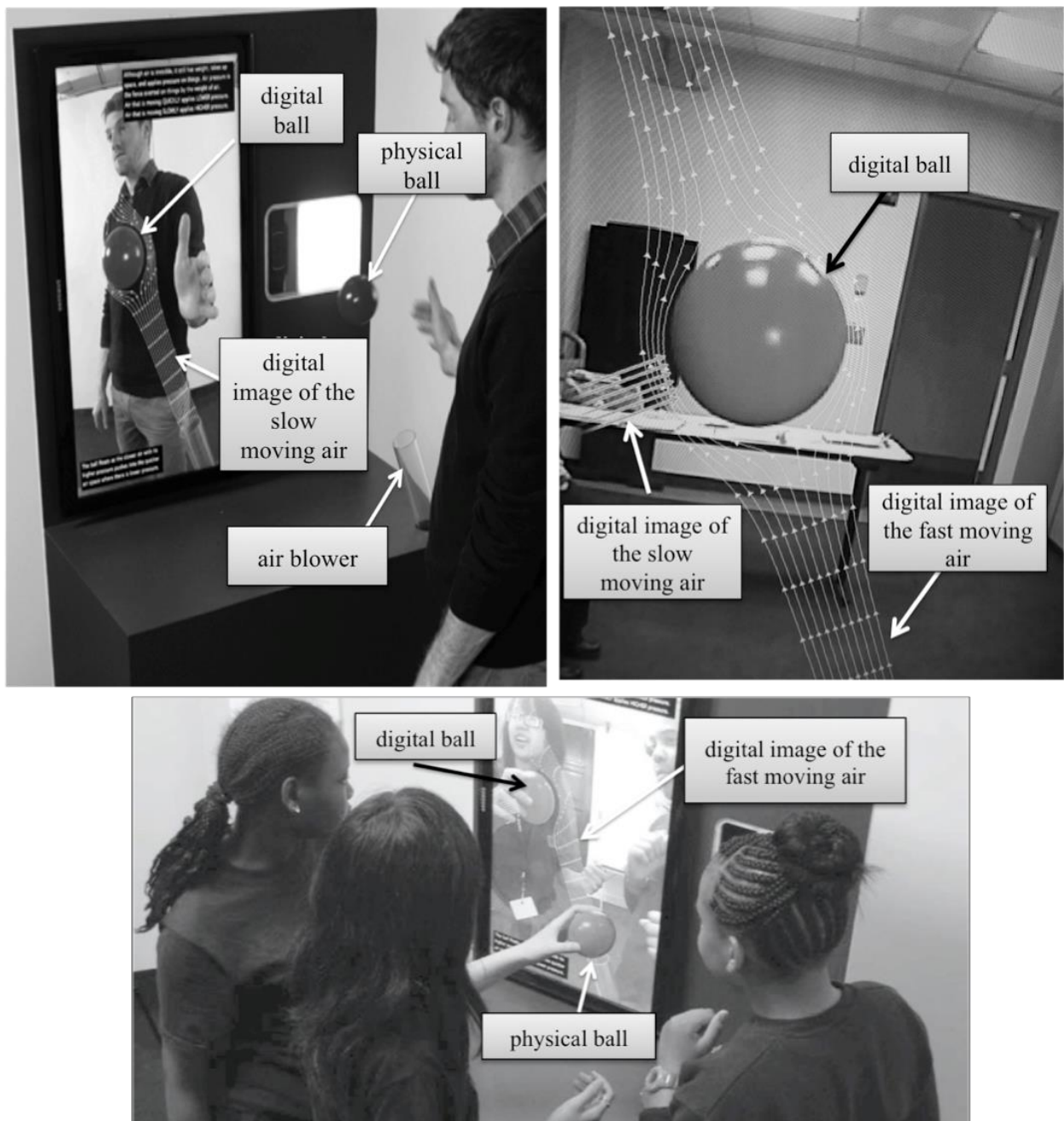
Figure 1. Images of the Bernoulli blower device with digital augmentation
